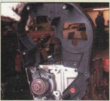
Remove the rear top timing belt cover, fitted with two remaining 8mm bolts – one at the front and one at the rear that goes into the water pump housing.
