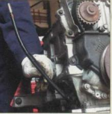
Remove the engine oil dipstick tube. This is fitted with two 8mm bolts at the base and one 13mm bolt for the steady bar bracket. Renew the gasket fitted – this has been known to leak oil.
