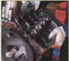
7 Remove the 8mm bolt from the top rear half of the timing belt cover. This will enable the cylinder head to be removed. Crack from the inside out, the ten Torx E12 head bolts. Store in sequence if you want to re-use them (see Rebuild Tips) and remove the head.
