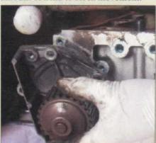
Undo four 8mm bolts for the water pump and one 13mm bolt which includes a locator for the timing cover. The water pump may need a gentle tap with a plastic hammer to break its seal to the engine block.
