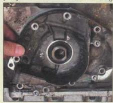
Remove the oil pump, fitted with nine 8mm bolts. All bolts are of equal length, except for the one fitted at the top left. Renew the gasket and rubber o-ring oil seal. To dismantle pump if required, undo two Torx screws underneath the gasket.
