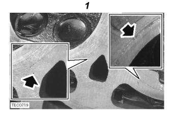
• Look for any sign of an indentation made by the bore eyelets of the head gasket. If there is an indentation from any of the four bore eyelets, the head has been overheated and the heat treatment properties of the cylinder head casting has been lost. The cylinder head must be replaced.
