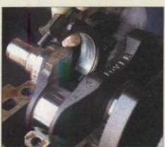
Remove one conrod cap at a time (10mm bihexagonal nuts), store in position fitted.
