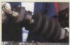
20 With all of the pistons removed, the crankshaft can be lifted out. Collect thrust washers from number three, engine block side.
