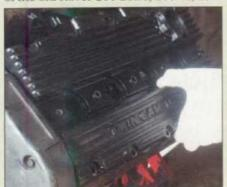
Remove the camshaft cover. This is fitted with 15 8mm bolts. Renew the gasket. When refitting, do not over tighten these bolts as they will damage the alloy camshaft carrier.
