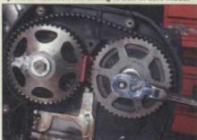
Fit a camshaft locking tool, making sure the markings on the exhaust cam are horizontal and a marking on the inlet cam pulley is horizontal to the exhaust. Crack the 17mm pulley bolts at the front and remove. Slacken the rear camshaft bolts, but don't remove yet.
